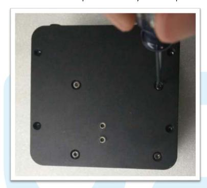
10. Fasten the bottom plate with top cover by screws x 4pcs
