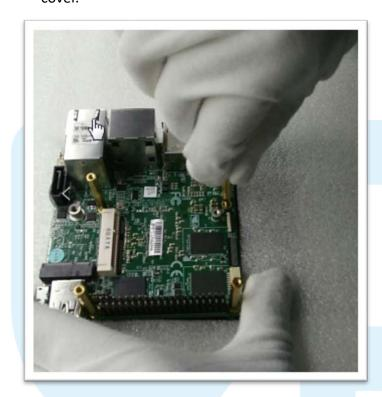
8. Place the board into the middle case, check well with the 4 sides exactly that match the IO sides.
