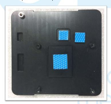
3. Peel of the blue protection film of thermal pad
