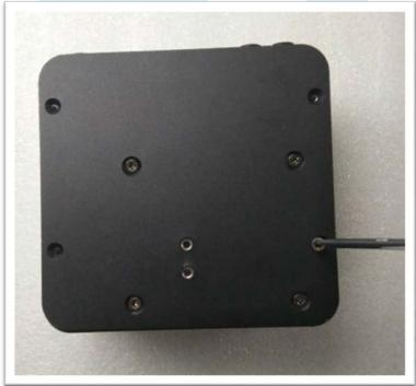
age e gap 11. Fasten the Vesa Mount with pre-assembled case by screws x 2pcs
